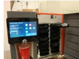
**3** On the dispenser remove the ingredient cartridge from the dispenser and insert a flush tray.
